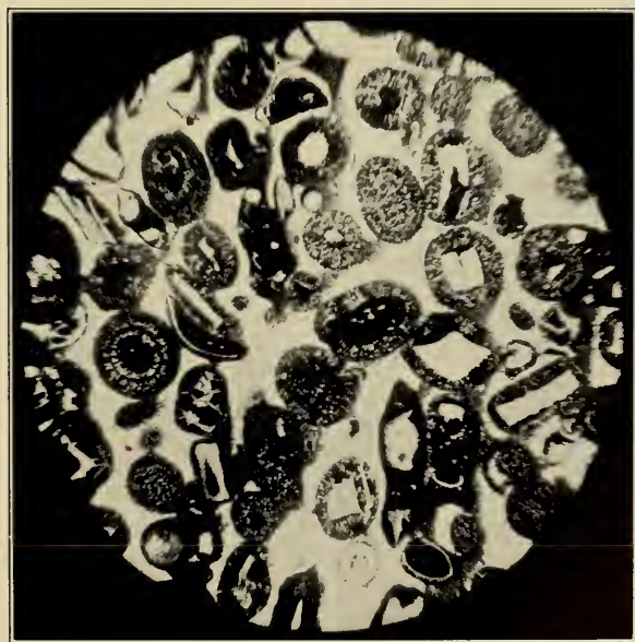
PLATE LX.—Photomicrograph.—Pink- or dove-colored oolite, Union Limestone, x about 20. (Photo. by A. Berg and W. E. Rumsey).
